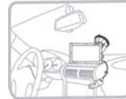
Insert DC plug of Cigarette lighter lead into the fused +12V socket of main system and connect the other end to the +12V cigarette lighter socket.
