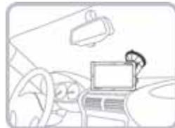
Slide the main system onto the mount clip and adjust the angle properly.
