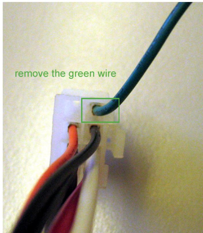
For this purpose you will need a long and thin tool for being able to press in the small „feet“ as shown on the pictures below :
